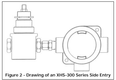
from the electronics housing via a  $\frac{1}{2}$ " NPT threaded cable entry point. The electronics housing is manufactured from aluminium alloy, with mounting lugs to provide a secure means of locating.
