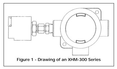
The manifold is manufactured from 316 stainless steel and protrudes from the electronics housing via a  $\frac{1}{2}$ " NPT threaded cable entry point. The electronics housing is manufactured from aluminium alloy, with mounting lugs to provide a secure means of locating.
